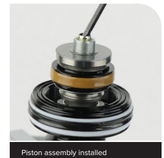
Piston assembly installed
