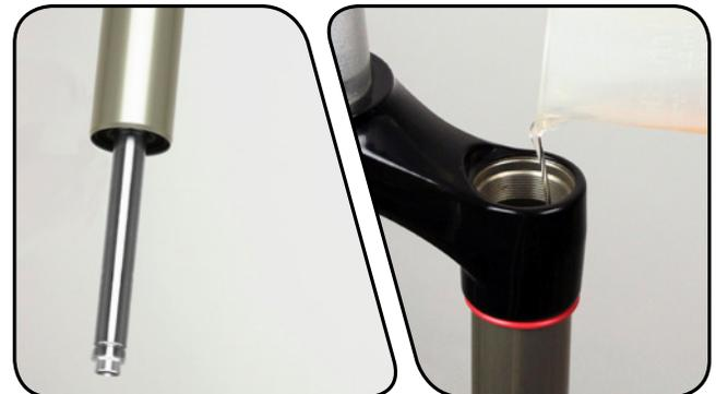
**11** Turn the hex shaft to the unlocked position. Insert the compression damper into the upper tube. Press down and rock side to side until the damper is installed.
