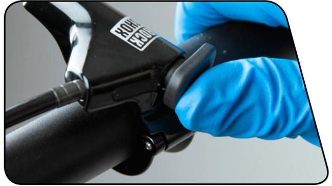
**2** **RLT:** Use a 2 mm hex wrench to loosen the cable pinch bolt on the spool and pull the cable out of the cable end slot. Use pliers to remove the cable end.
