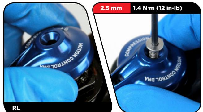
**Remote Only:** Install the cable stop collar onto the top cap with the cable stop facing toward the front of the fork, perpendicular to the crown. Use a 2 mm hex bit socket to tighten the collar clamp bolt to 1.4 N·m (12 in-lb).
