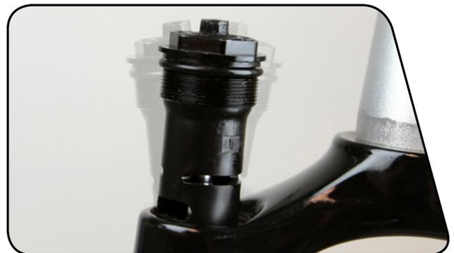
**12** Use a torque wrench with a 24 mm socket to tighten the compression damper to 7.3 N·m (65 in-lb).
