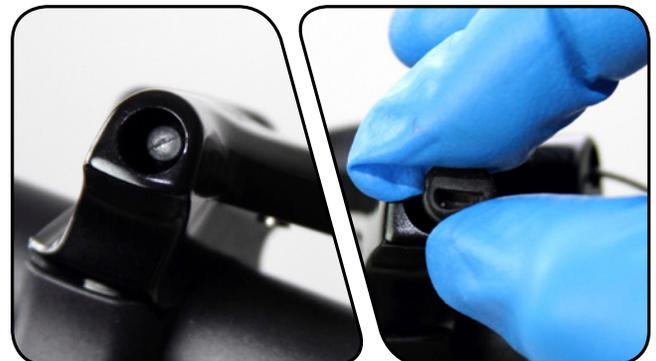
**4** **RLT:** Wrap the cable around the spool and insert it through the cable fixing port. While firmly pulling the cable, use a 2 mm hex wrench to tighten the cable pinch bolt to 0.9 N·m (8 in-lb).
