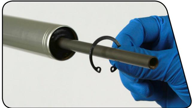
**6** Firmly pull on the air shaft to remove the air shaft assembly from the upper tube. Clean and inspect the assembly for damage.
