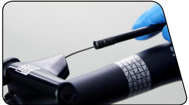
**4** Use a 2 mm hex wrench to open the cable hatch cover. Push the cable through the remote until the cable head is far enough out of the lever to access.
