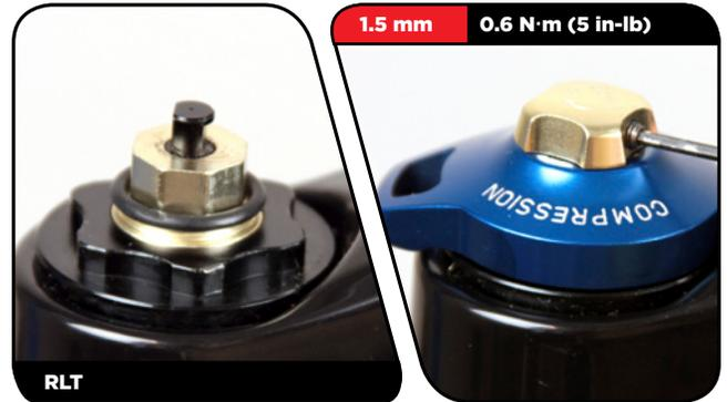
**RL:** Install the compression adjuster knob with the knob dial against the hard stop.
