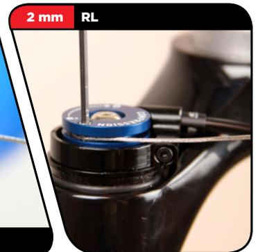
**3** Disconnect the cable from the damper and pull the cable housing off the cable.
