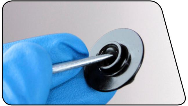
**5** Place the tips of large internal snap ring pliers into eyelets of the snap ring, located at the bottom of the non-drive side upper tube. Press firmly on the pliers to push the air shaft guide into the upper tube enough to compress and remove the snap ring.
