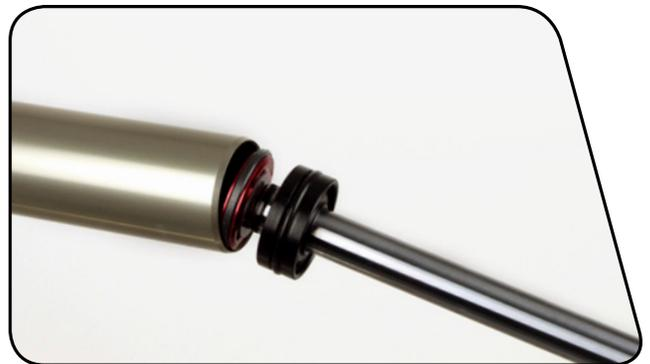
**8** Push the rebound seal head firmly into the upper tube until the retaining ring groove is visible.
