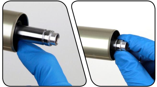
**9** Use internal snap ring pliers to secure the snap ring into the retaining ring groove.
